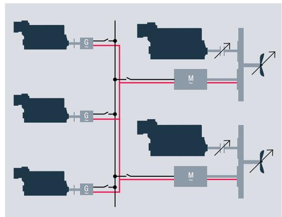
Example: Navy vessel using electric propulsion for slow sailing speeds
