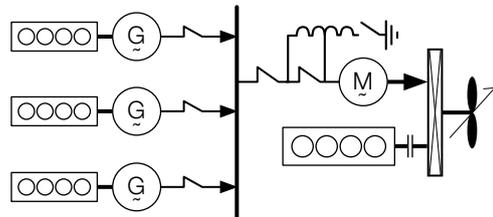
*b) Installed genset capacity is in the same range like the PTH-motor power rating ("Weak mains")*
